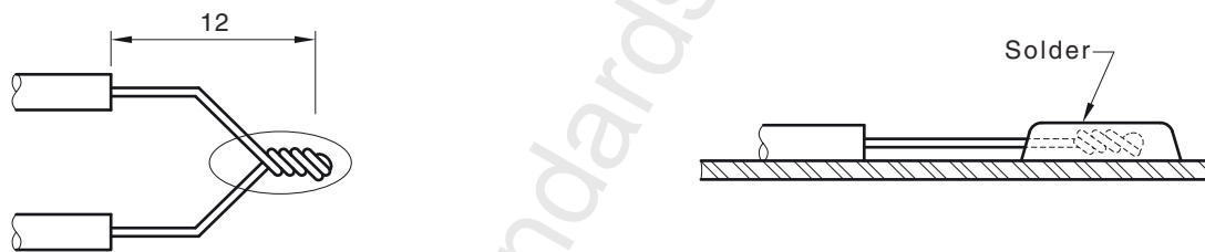
(c) Thermocouple soldered to metal surfaces
